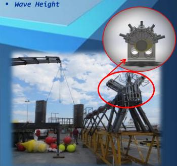
This pump has developed maximum power of 7kW, with waves of 0.65 m and 400 l floats.
